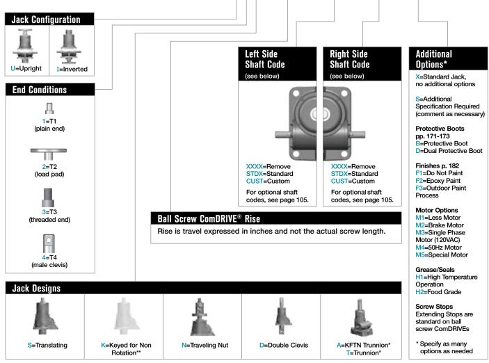
\*Standard trunnion mounts available on 2-ton through 20-ton jacks. (See page 183) \*\*Keyed for non-rotation is not a standard option. Contact Joyce.
